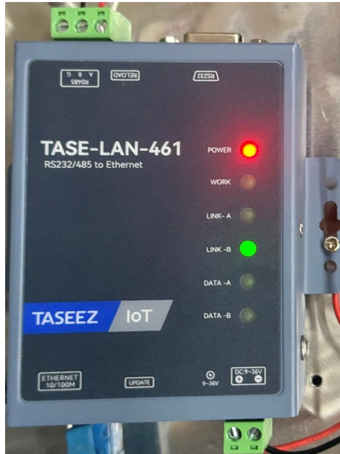
Figure 18. Device Connected to Modbus TCP Client
