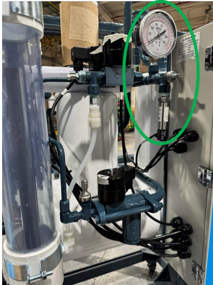
Figure 9. H9490 and Pressure Transducer Installation
